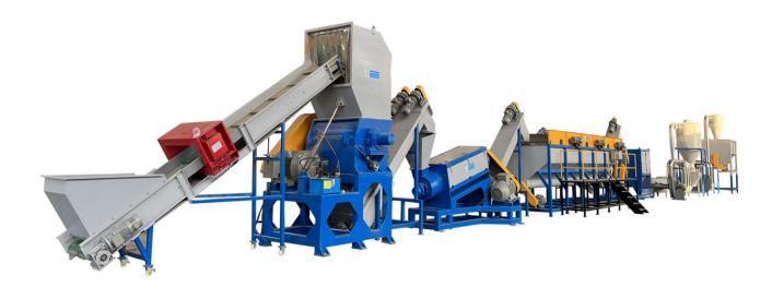
Plastic PE PP film bag washing recycling line is used to processing and washing post-consumer LDPE film,LLDPE film,PP woven bag,etc. The vital point of PE PP film washing recycling solution is how to improving output capacity and control the final flakes humidity.RETECH technical team always pursue this responsibility to make it happen.
